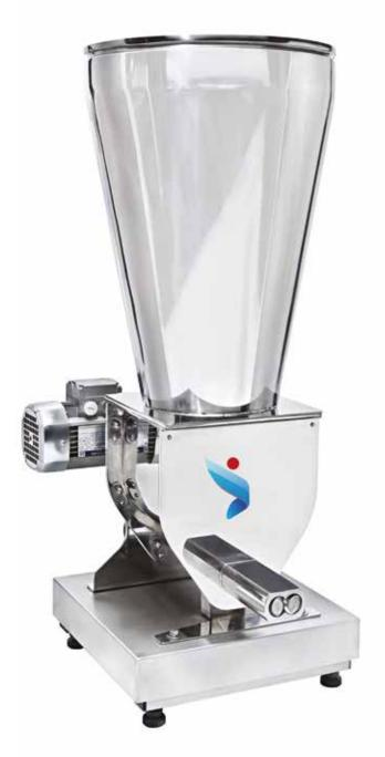
When in addition to precision a high consistency of feeding is required, it is necessary to use a twin screw system. The D Series feeders, equipped with twin extraction screw, ensure a homogenous material flow due to the particular machine process, that ensure a perfect coupling. The D Series twin screw feeders are designed for feeding materials in powder and synthetic fibers and are especially recommended for very fine powders.
