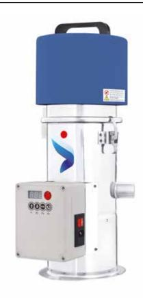
The single-phase loaders CMP are indispensable components for the feeding of different types of granules and reground materials in the complex plastics processing systems. These loaders are adopted for receiving free flowing powders pneumatically that are extremely fluid with bare density smaller than 0.8kg/dm3. Their application is limited to flow rates of less than 300kg/h with a transfer distance of less than 15mt.
