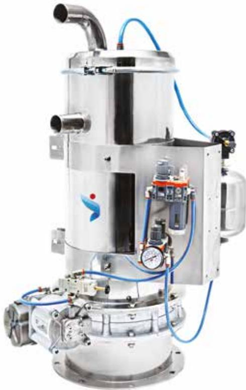
The Single-phase loaders CTM series are adopted for receiving free flowing powders pneumatically (suction) that are extremely fluid with bare density greater than 0.5 and smaller than 1.2kg/dm<sup>3</sup>.
